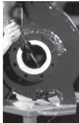
Fig. 5: Electric spark testing of an isostatically processed Teflon PTFE pump housing.
